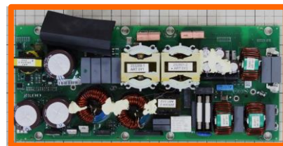
Power stage board
