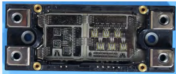
Module after removal of the control board
