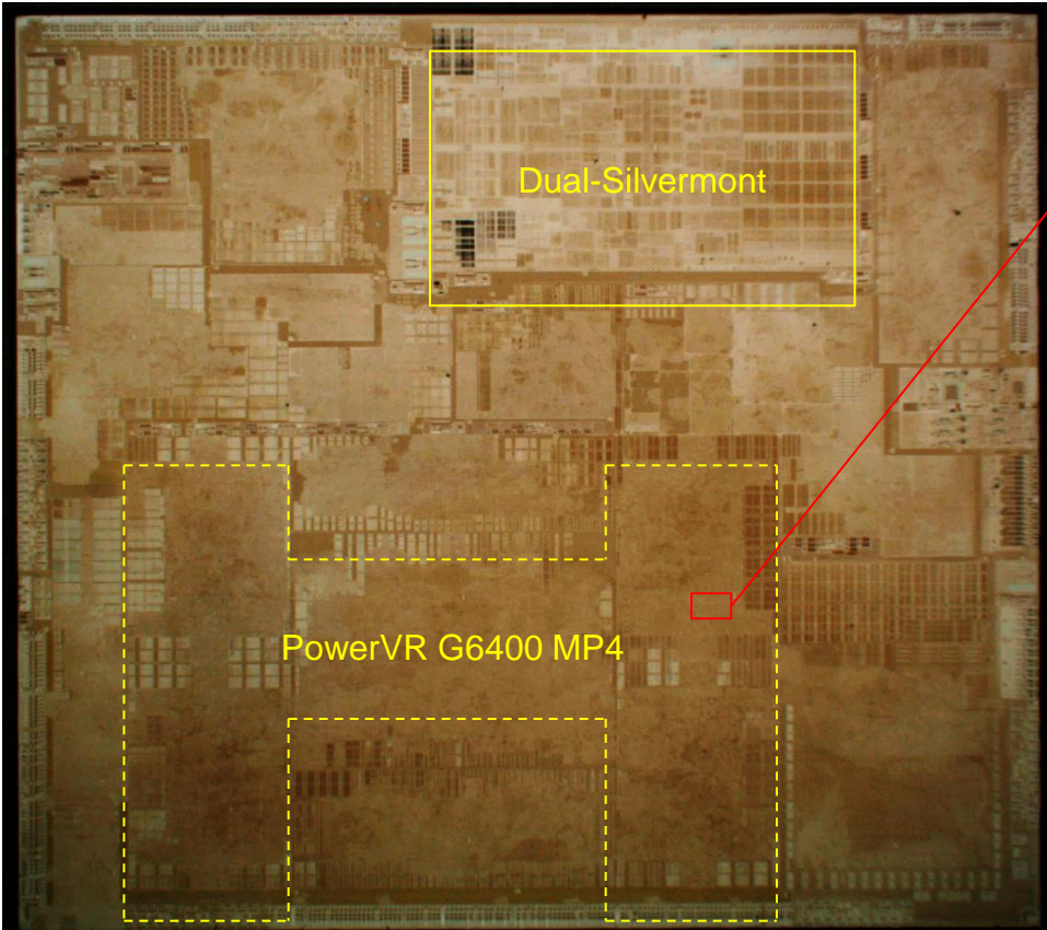
Fig. 5-10-1 Die Top-View (Diffusion layer) 1mm
