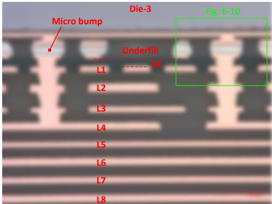
Fig. 6-9 Micro-bump cross-section image
