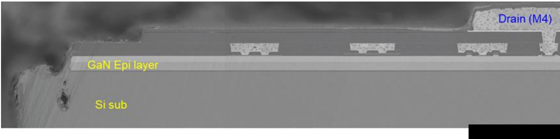
Die edge Cross section SEM image
