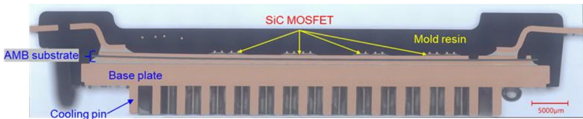
Module Cross-section OM image
