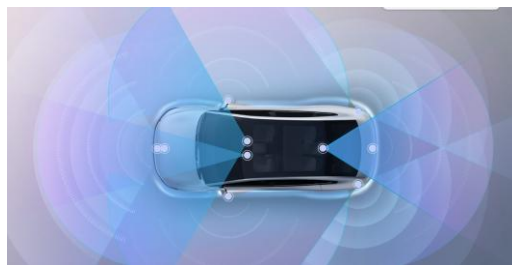
22pcs of ADAS sensors and Orin chip
